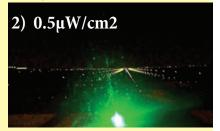
2) FAA Simulator Study, level 1 (10 times greater than FAA Laser-Free Zone level). Roughly equal to bright startle or distraction. 5mW laser pointer at 3,700 ft. **Runway partially obscured.**
