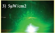
3) FAA Simulator Study, level 2 (FAA Critical Flight Zone), where glare is the primary hazard. 5 mW pointer at 1,200 ft. **Runway mostly obscured**.
