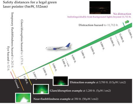
Figure 2: "Safety distances for a legal green laser pointer (5mW, 532nm)"
